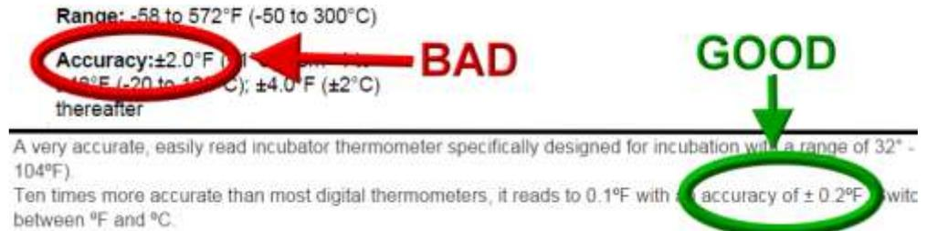
**CAUTION:** All digital thermometers appear to be accurate but **most** are grossly inadequate for incubation. A digital thermometer **must be calibrated** and **must have a sensitivity** of no less than  **$\pm 0.2^\circ$  F**.
